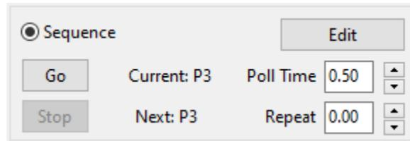
The sequence section allows the user to poll a number of register addresses in sequence.
