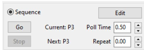
In the main window, when a current sequence is defined, the polling can be started/stopped with the “Go” and “Stop” buttons. The “Go” will be greyed out and unable to press if no sequence is defined. The “Poll Time” value is the time between polls. The “Repeat” value is the time after a sequence has completed till it starts again. These values can either be edited using the relevant up and down arrows or by typing a value in directly.
