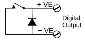
Each digital output can be considered as the contacts of a relay with a reverse clamp diode.
