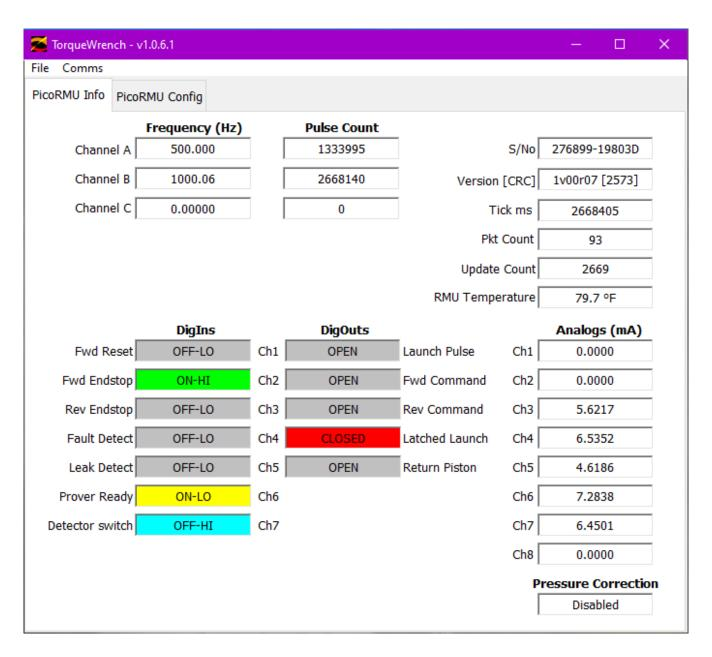
If serial data is received using the PIU protocol, TorqueWrench will add the labels for both the Digital Inputs and Digital Outputs, as shown in the screenshot above.
