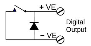
When the digital output is **OPEN** no current will flow from the +ve to the -ve terminals. When the contacts are **CLOSED**, current will flow as long as the correct polarity is observed.
