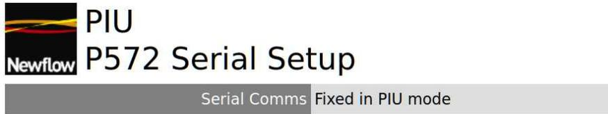
In PIU mode, the serial communications are preset to match the default settings for PROVEit and cannot be altered.
