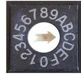
This defaults the Modbus Slave address to Address 1 on both the two serial ports (running Modbus RTU serial) and the Ethernet port (running Modbus TCP).
