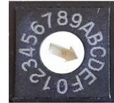
This defaults the Modbus Slave Address to 1 on both the two serial ports (running Modbus RTU serial) and the Ethernet port (running Modbus TCP).
