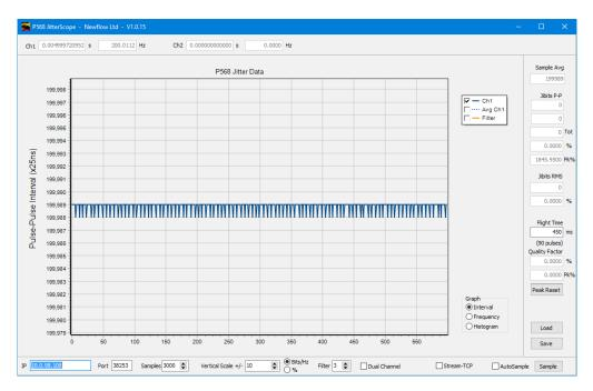
In the screenshot above, the input frequency is about 200 Hz so although 3000 samples are requested, the P568 will stop data acquisition after 3 seconds, hence only collecting around 600 samples.
