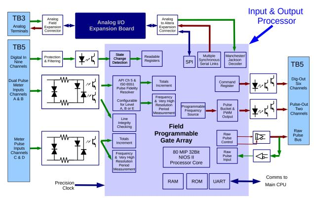
All of the specific hardware listed above, together with the asynchronous serial ports, the program storage, working RAM and the NIOS II 32 bit processor have all been designed and compiled to fit within a single Intel/Altera field programmable gate array. This device is known as the I/O Processor. The NÅNOconf software allows users to load new or different versions of the Intel/Altera program, so that the I/O can be infinitely reconfigured, if so required.
