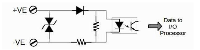
From an operation perspective, each digital input can be considered as a light bulb with series diode. The voltage must be applied in the right polarity but, because they are all individually isolated, the installer has freedom to connect them in a number of ways.
