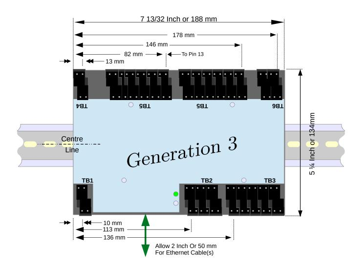
The highest point of a NÅNO mounted on a din rail will be 2¼ inches (56mm) above the mounting surface, but note, the Field wiring emerges vertically, and we recommend at least 2 inches (50mm) of clearance above the unit for the cables. If cable tags are used, then allow additional height, as the bend radius is increased.
