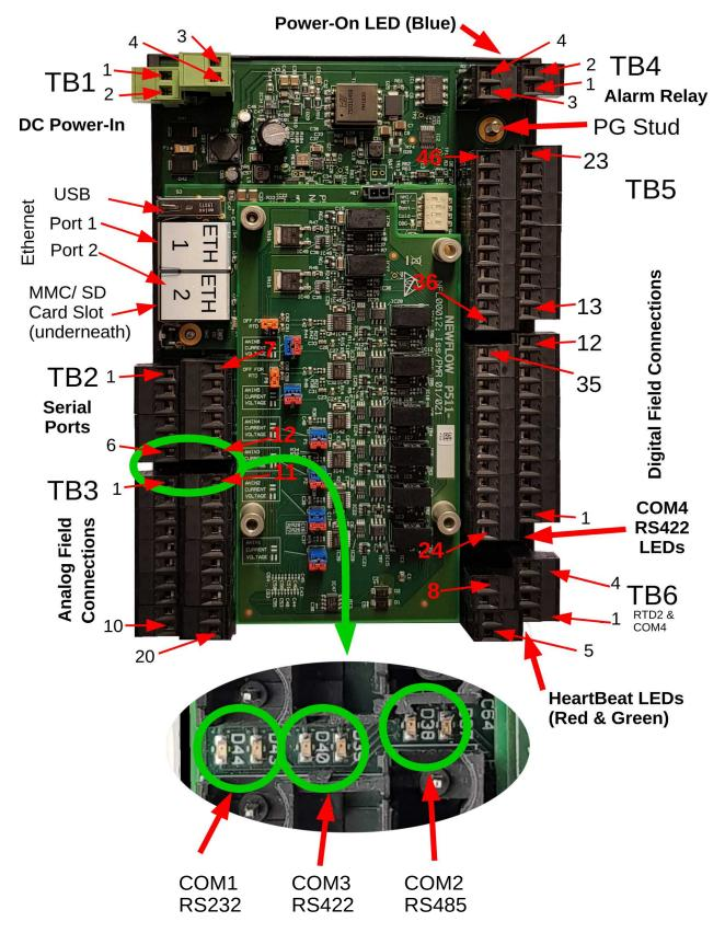
**NOTE:** The communication tell-tale LEDs for COM1, COM2, COM3 & COM4 show RED for data transmitted from the NÅNO and GREEN for data received by the NÅNO.
