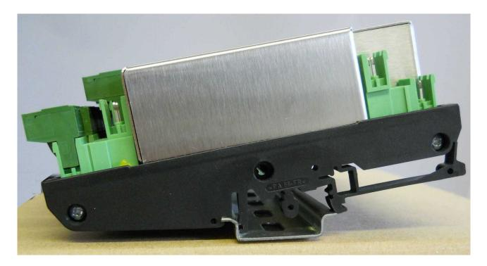
To remove the unit, apply a small flat-bladed screwdriver into the release slots as illustrated and lift the front.
