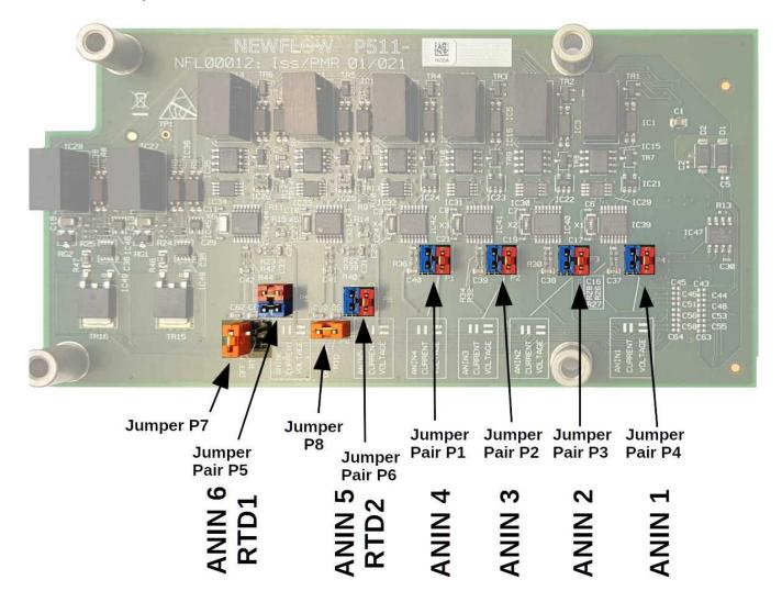
**NOTE:** In the photograph above, AnIn1 to AnIn5 are in 4-20mA current mode and AnI6 is in RTD mode
