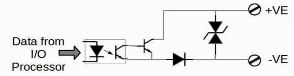
There are six Digital Outputs provided. Each Digital output has a high current Darlington output which is surge and reverse connection protected. Each output is Galvanically isolated from all other I/O points. This allows it to be connected to either the positive rail to act as a current source or connected to the negative rail to mimic a grounded open collector output.
