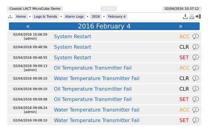
If the entire Alarm history is needed, it can be retrieved using the XML communications for routine and regular use, but for immediate access, the data can be downloaded from the LACT-Pro® controller website, simply by clicking on the Download Icon, at the top of the screen. The data will be downloaded as a single file in Tab Separated Variable (.TSV) format and can be opened and manipulated in OpenOffice, Excel or other spreadsheet programs.
