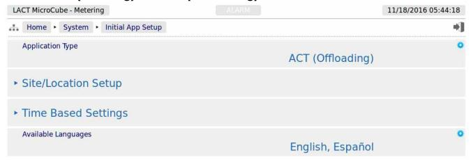
The first line, showing the data point *Application Type* needs to be configured before any further settings are made.
