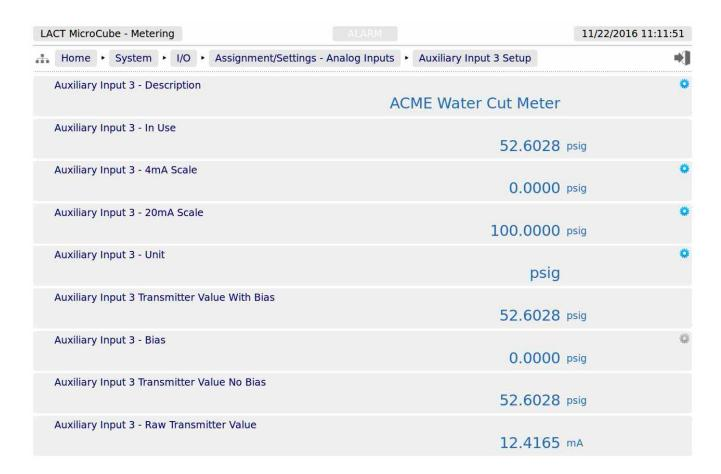
This Auxiliary input is being used to test another vendors water cut meter. The performance of the alternative meter is monitored by using the information from the data logger, either from the Trending Display, or by downloading the information from the data logger.
