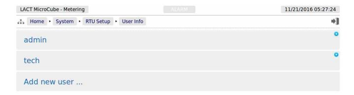
User details can be viewed by clicking on the relevant line containing the gear icon. Clicking on the *admin* line opens the Edit Value dialogue box, and you can change the name and password, but not the
