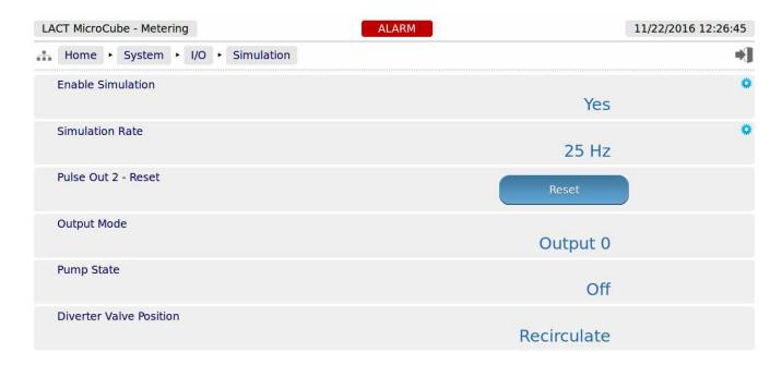
The simulated pulse rate is programmable in 8 steps between 10 Hz and 500 Hz.
