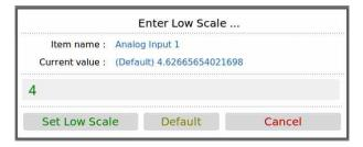
This has pre-loaded 4.0mA into the low scale field. It is not yet being used and will not become active unless confirmed at the end of the process.
