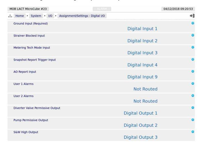
**NOTE:** The LACT-Pro® application does not check for exclusive assignment of any I/O points. It is recommended to record any changes to the I/O using the I/O schedule drawings available in <u>Section 12 I/O Schedules</u>.
