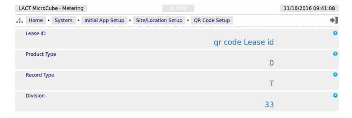
The QR Code Setup information can be used for any purpose, but Lease ID and Record type are text fields, up to 32 characters.
