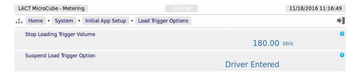
**NOTE:** If the **Load Trigger Options** sub-menu is not shown, the LACT-Pro is in ACT (Offloading) mode, rather than LACT (Loading) mode.
