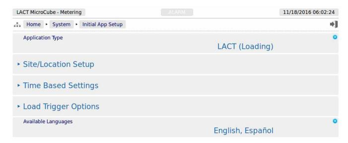
By selecting the LACT (Loading) option, a sub-menu for the Load Trigger Options has been made visible. Clicking **Site/Location Setup** sub-menu will show the screen below.
