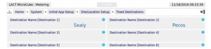
The screenshot above just show a part of the menu, 15 Fixed Destinations are supported. The destination can also be configured remotely using the XML communications.
